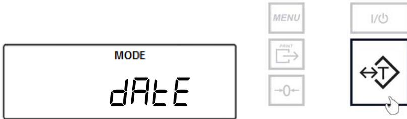
3. Press the T key to scroll between the month and then the day. Press the zero key to increment a digit.
