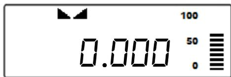
**Note: Re-zeroing the scale will reduce the capacity of the scale by the re-zeroed weight. The remaining capacity is displayed as a percentage on the right side of the display.**
