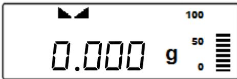
3. When weighing, always place the mass in the middle of the pan. The weighed result may be taken when the stabilization indicator reappears on the display.
