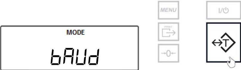
2. Choose the baud rate to be used (“1200”, “2400”, “4800”, “9600”, “19200”, “38400”, “57600”, and “115200”). To confirm the selection, press the T key.
