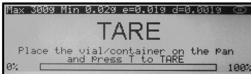
2. Place a vial or a counting container on the pan. The container weight will be displayed.
