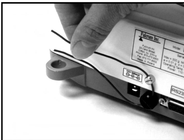
2. The seal may then be placed over the wire. Do not attempt to remove the calibration screw as it will rip the wire and break the seal.
