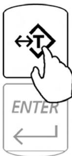
4. The display will show a dotted line which indicates the scale has begun the taring process.
