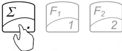
Once the sigma key has been pressed, the scale will display the current recipe. The recipe can be saved in the scales permanent and electronically erasable memory.
