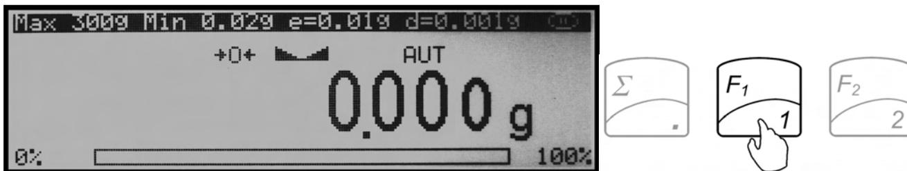
3. When weighing, always place the mass in the middle of the pan. The weighed result may be taken when the stabilization indicator appears on the display.
