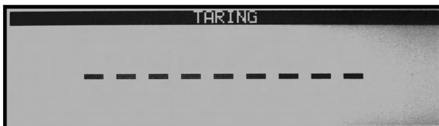
4. When finished clearing the tare, the scale will return to Weighing Mode.
