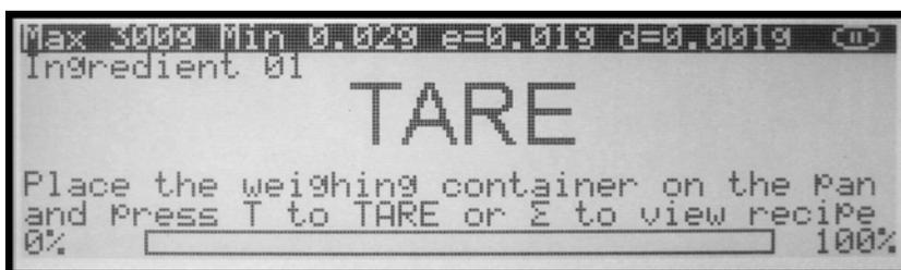
3. Place a container on the pan and tare it by pressing the T key.
