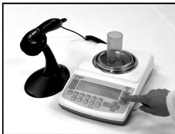
**Note:** Minimum individual piece weight allowed is 30mg (3e). With a sample size of 10 pieces, the sample weight must be equal to or greater than 300mg (30e). Attempting to set a sample size of 10 pieces with a total sample weight which is lower than 300mg (30e) will result in an error.
