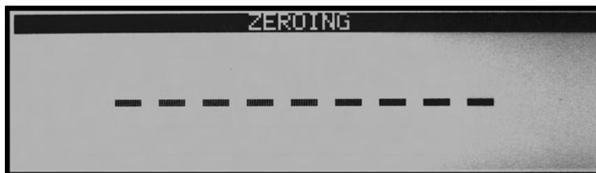
5. When finished re-zeroing, the scale will return to Weighing Mode and the display will indicate 0. A new center of zero has been set, and the scale is ready for weighing.
