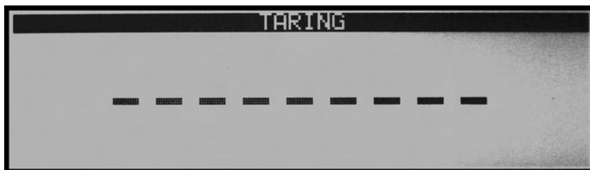
5. When finished taring, the balance will return to Weighing Mode. The display will indicate 0, and the NET indicator will be shown on the display signaling the next weight taken is a NET result.
