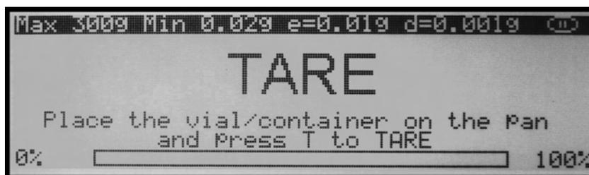
3. Place a vial or a counting container on the pan. The container weight will be displayed.
