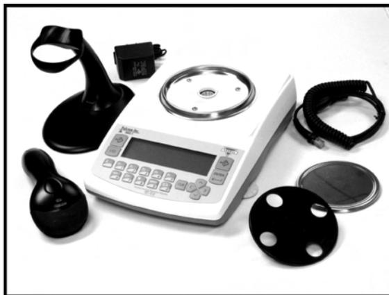
2. After removing the pan base and the pan from their packaging, carefully install the pan base onto the scale by placing it on the pan support located in the middle of the scale. Once the pan base has been installed, gently place the pan on the base as shown below.
