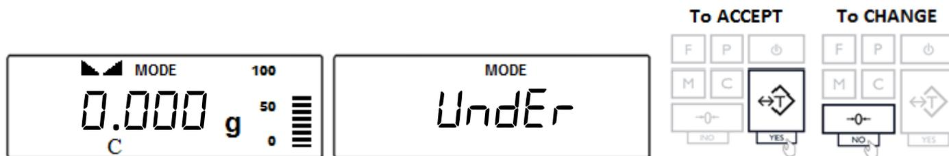
**Note:** The *UNDER*-limit displayed will be from the last time the function was used. If this is the first time the Check Weighing function is used, the limit will be set to 0.000g.
