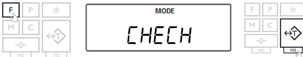
2. The current, set *UNDER*-limit and the command “*Under*” will appear on the display sequentially. To accept the current *UNDER*-limit, press the “T” (Yes) key. To change the limit, press the “→0←” key.
