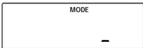
3. After setting the *UNDER*-limit, the current, set *OVER*-limit and the command “*Over*” will appear on the display sequentially. To accept the current *OVER*-limit, press the “T” (Yes) key. To change the limit, press the “→0←” key.
