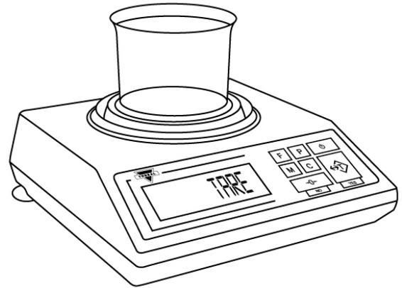
5. The scale is now ready to use. To perform check weighing place your object on the pan to check whether the weight of the object falls within the designated range. If the weight is less than the lower limit the scale will display the weight of the object and the command “UndEr”. If the weight falls within the range, the “ACCEPt” command will be displayed. If the weight exceeds the upper limit, the scale will display “OvEr”.
