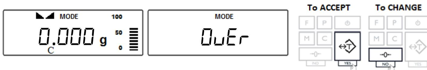
4. Once both limits have been set the scale will display “tAr-E”. Place a container on the pan and press the “T” key to tare.
